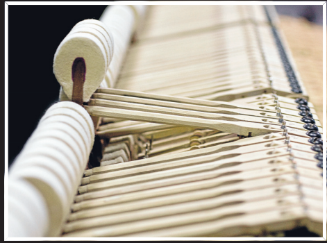
Top heavy: The hammers that strike the strings.
